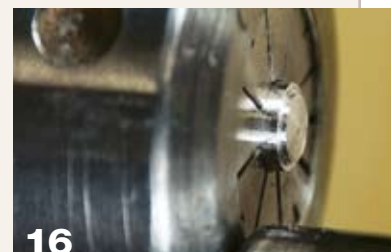
Turn a 0.335" tenon about 0.020" wide in the insert.
