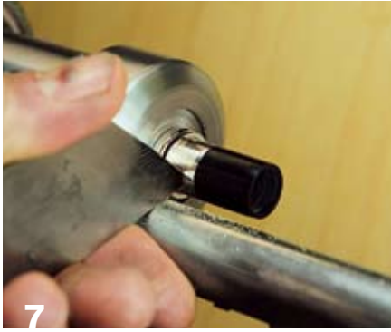
7 With a scraper or parting tool, reduce the centerband fitting for a slip-fit.
