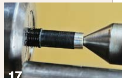
Grip the El Grande section in a collet, add the little support disk, and use a live center in the dimple. Turn away the contoured grip to a .335" diameter for a slip-fit Broker tube.
