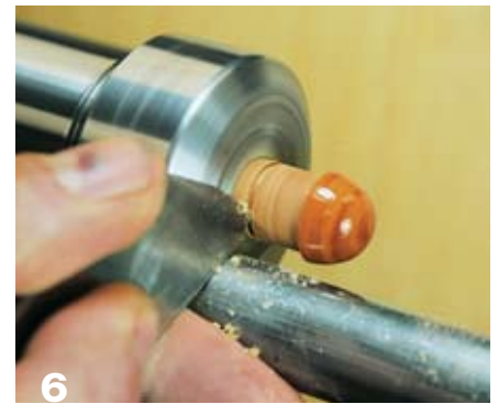
6 Part off the finial cap, leaving a \frac{1}{2} "-long tenon.
