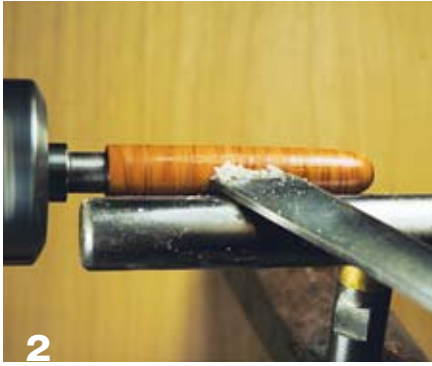
2 With an old skew gently scrape cured cyanoacrylate (CA) from the body.
