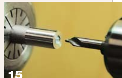
A centering drill is ideal for drilling aluminum rod.
