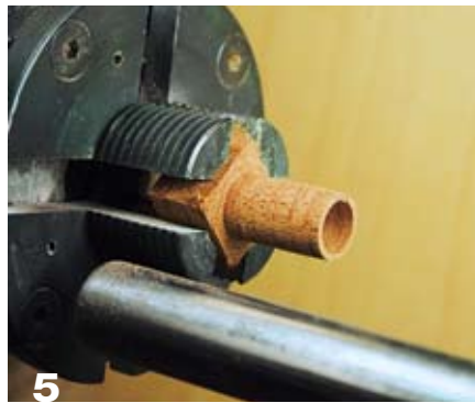
5 Reduce the diameter to \frac{7}{8} ", which will slip into the cap brass tube.
