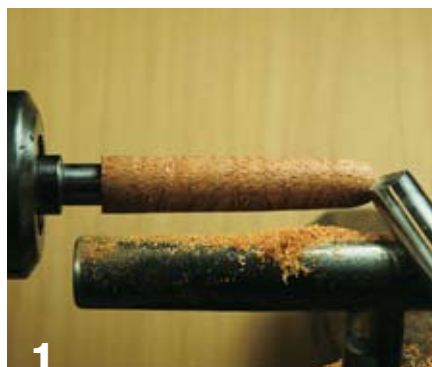
With a ½" spindle gouge or 1" skew, turn the pen barrel with a rounded end.
