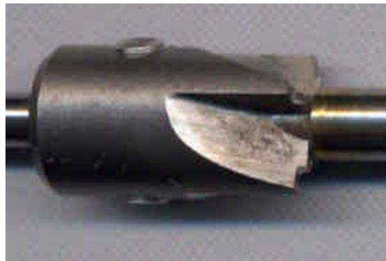
a metal lathe, using a Dremel flex shaft held in the tool holder as a cheap tool-post grinder.) After I cut a recess pocket into the upper end of the cap, I use a small grinding stone held in a Dremel tool to cut a slot for the clip to exit.
