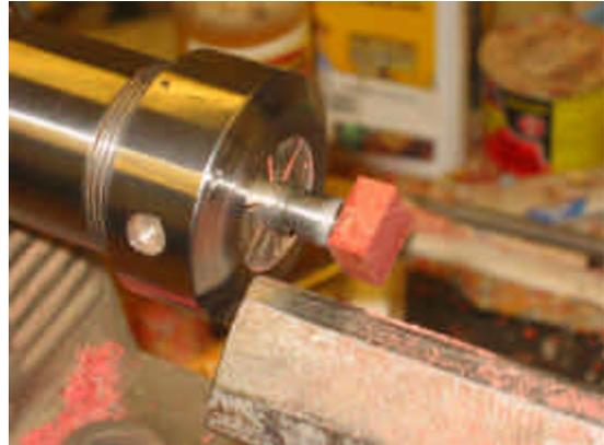
10 seconds with the spindle gouge transform the square into something that resembles the finial. I am just turning to a cylinder basically, rounding it over slightly, just hogging of material staying outside the desired shape.
