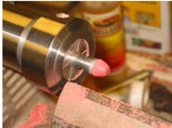
Now I turn the final shape. I like using a pyramid tool from Crafts Supplies for that, because it lets me swing the whole arc without having to reposition the tool rest.
