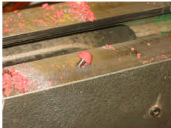
Using this finial on a Euro turned from a Slimline pen poses another challenge. The Slimline clip must be recessed into the body of the cap or there will be an unsightly gap between cap and finial. I modified a pen mill to cut a .333" diameter recess. (I shape the cutter on
