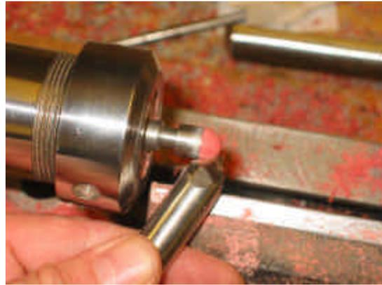
The nice thing is I can unscrew the finial any time and try it on the pen, coming back to the exact same position on the mandrel. This way I can make sure that not only the diameter matches exactly, but also that there is a nice smooth transition from the cap barrel to the finial without a break in curvature. Here it is, ready for finishing!
