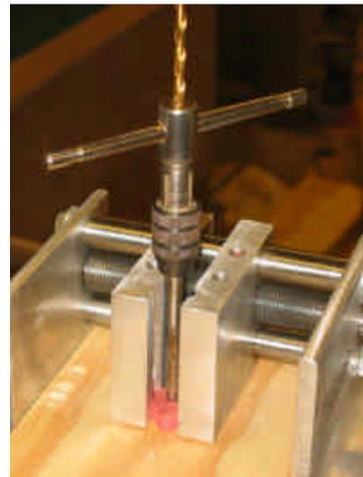
Now I simply screw the stud into the hole. You can use a drop of glue, it seems to work just fine without that also, but it may be a good idea if the pen undergoes climatic changes to assure that the finial does not come off. It is not necessary for the fabrication. I often use a finial adapter to give me a better handle on the stud while screwing it in.
