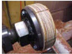
The faceplate is mounted on the lathe for truing and balancing.
