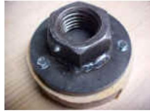
The faceplate is mounted to the wood block with the 3/4" #8 screws.
