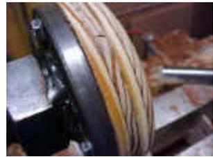
With no reason to be at exactly the same diameter as the steel on the faceplate, the wood is only turned until round and close in diameter.
