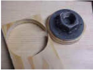
The faceplate is checked for fit and the best side of the plywood is used to seal to the faceplate.
