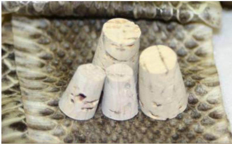
Now, let's move one. Corks are needed to close off the ends of the tubes. Now, let's move to the next step...preparing the tubes for casting. The major problem is to hold the tube off the bottom of the mold. Many things were tried and corks proved to be the best choice, for me and others, at least. Others may discover a better or easier way to do this. Anthony Turchetta explains how to cast skins using a two pour casting in his excellent article on PR casting.
