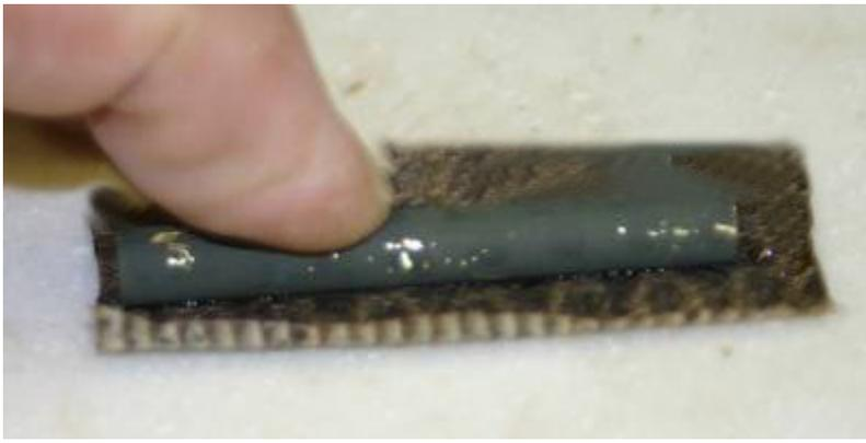
Set the tube on the glue bead and hold until set. Then roll the tube to one side and the glue will squeeze in front of it. Turn the tube/skin around and place another bead of glue next to the tube and roll it toward the end. Overlap this second edge over the first edge. Do not try a butt joint. The overlapping joint is the only one to use.
