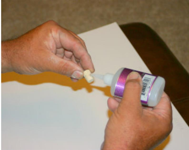
**Run a bead of medium CA around the cork and securely place it in one end of the tube. Fill with weights (remember, I use BB's), then CA the other cork and place it in the other end. Be sure the glue makes a good seal all of the way around the cork and the brass tube's end.**
