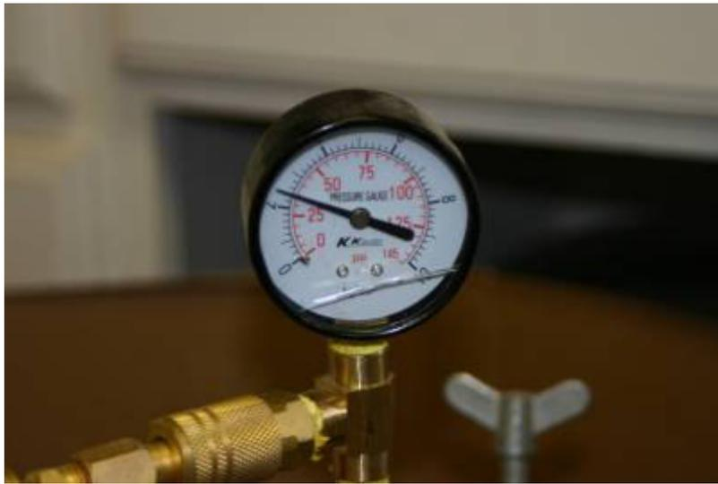
Before the vacuum step I was pressurizing the tank to 50 psi. Now that I degass the resin with vacuum, I've dropped the pressure back to 25-30 psi as indicated on the gauge in the next photo.
