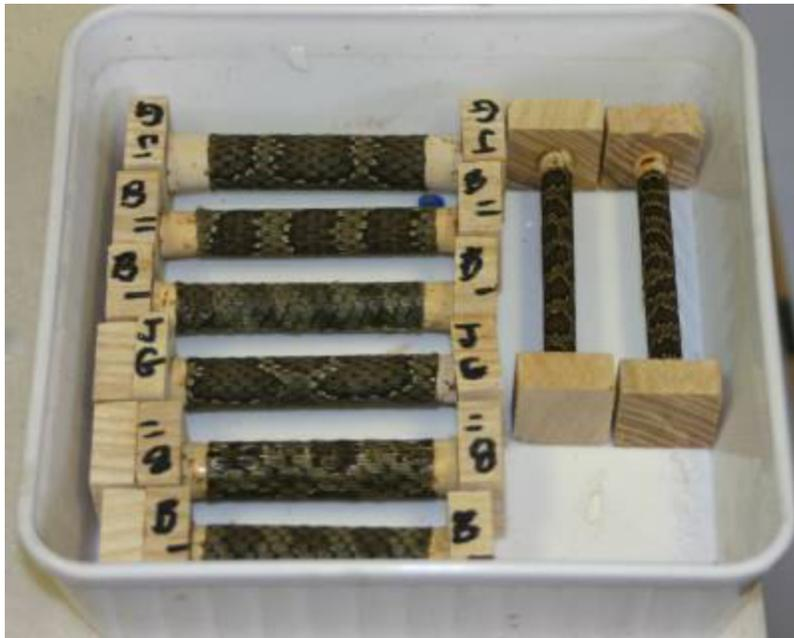
Here is my mold filled with tubes ready to cast. I identify the tubes to keep the pen pairs together. I cut the skin patches from adjacent areas of the skin and like to keep the skin matched on the same pen. I will leave the marking scheme for other casters to develop for themselves.
