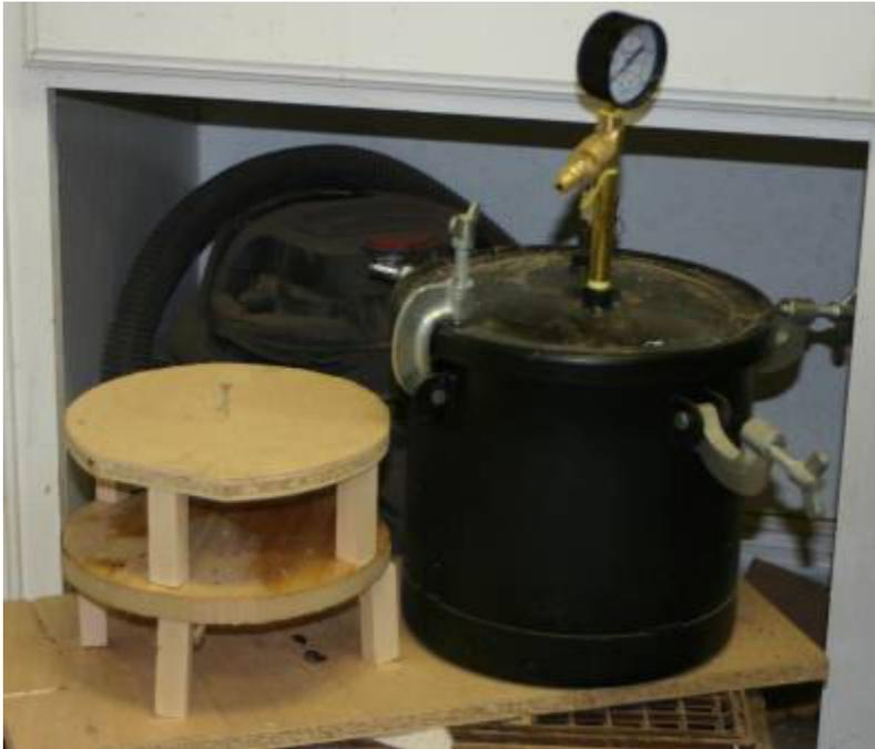
Also pictured are the two racks I use so I can cast two molds full of tubes at once. The bottom of the tank is concave and I place a round plywood disk in the bottom. This holds one mold; the second mold is placed on the next layer. I use a top plywood disk to keep the air from the compressor from blowing out the resin, although it may not be needed.
