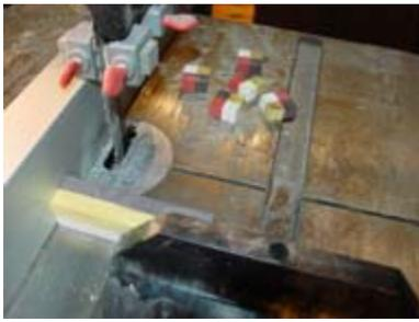
10) Sand each section on the freshly cut sides. I do this by hand with sand paper on a piece of glass to ensure the surface stays flat.
