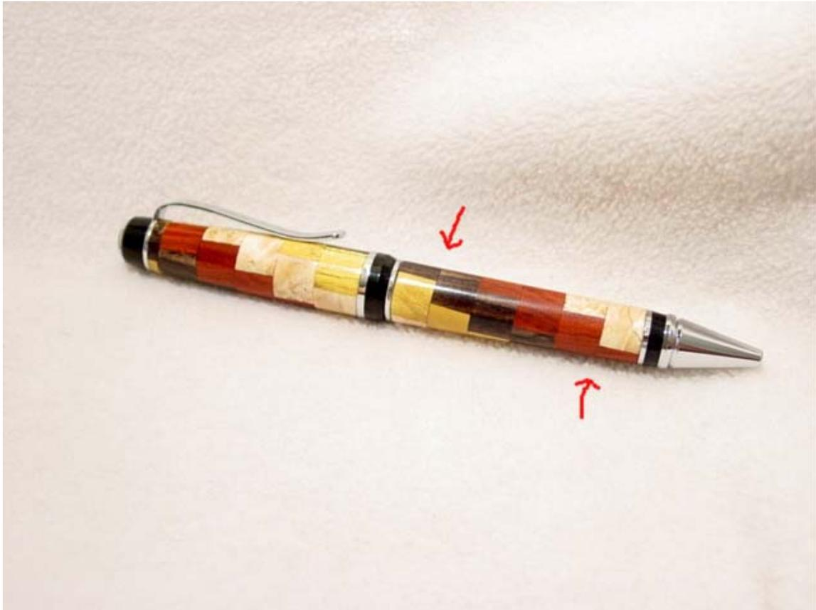
Another thing you can do with the process is to make a checker design. Just use two colors and instead of rotating the small sections 45 degrees, rotate them 90 degrees.
