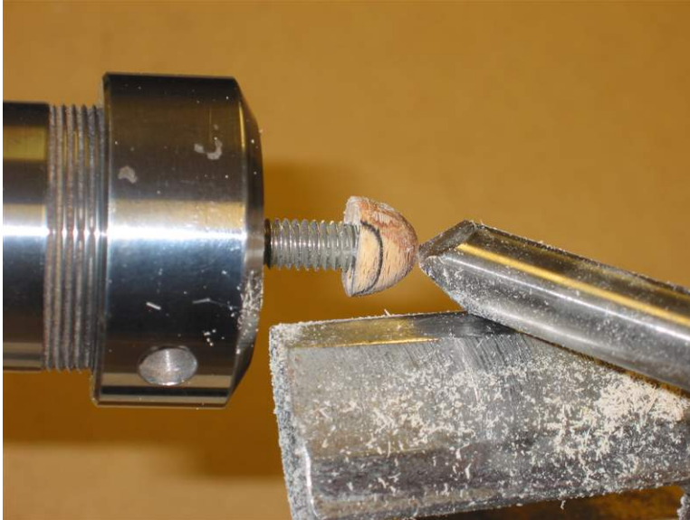
Picture 8: Turning the cap finial
