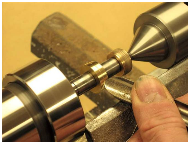
Picture 2: Brass can easily be turned with regular lathe chisels
