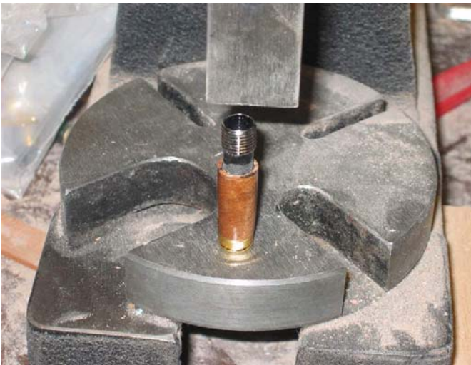
Picture 5: The nib ring is glued and pressed onto the plastic tube, the turned barrel is glued on, and the threads are glued and pressed on to complete the section
