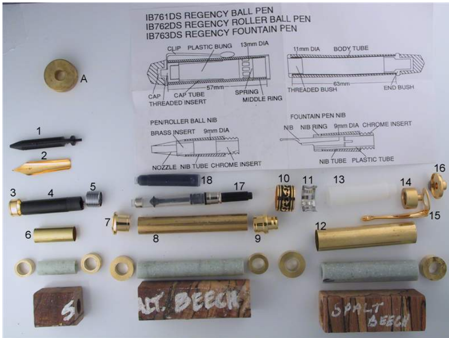
Picture 1: The items that come in the kit are labeled 1-18. Also shown are the 'instruction sheet', the shim tubes made from Corian, the sizing disks made from brass, an unturned sizing disk 'A', and the blanks used for this pen.
