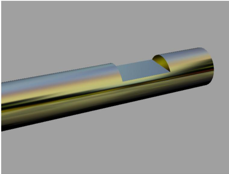
The depth of the flat has to be the same as a pin. It's best to make the pin first, out of steel or a cutoff nail even, then make the flat with a depth to match.
