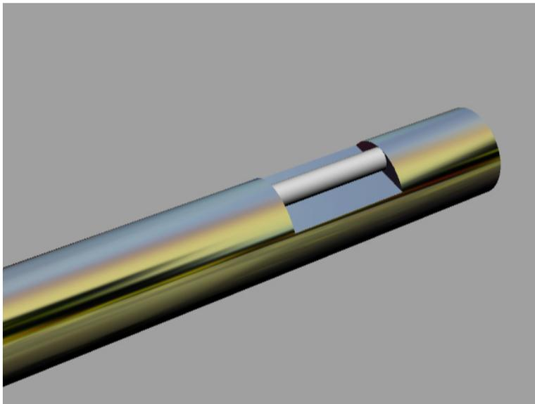
The pin is slightly shorter than the flat so it does not bind at the ends.
