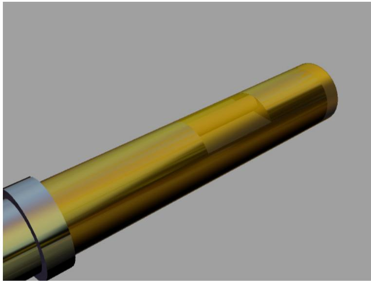
If you have a metal lathe you can add a sliding bushing, although I prefer not to. I work with calipers, and I find having the end open gives me an easy way to square the barrel with a parting tool.
