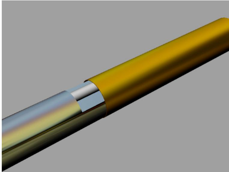
When the tube is slid all the way on, you can twist it slightly (against the rotation of the lathe) and the loose pin will act like a cam and lock the tube in place.
