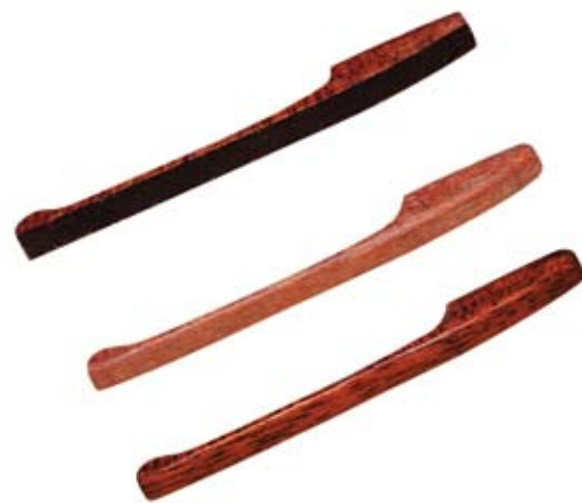
From the top: A blood wood lasered clip with burn marks ( top ), sanded ( center ), and finished with a thin coat of CA glue ( bottom ).
