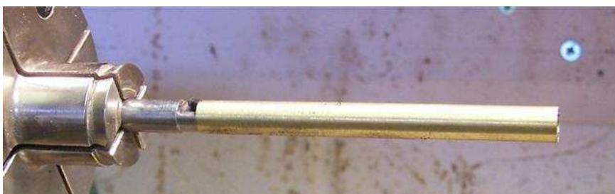
Here you can see why I didn't cut the threads off. I tapped an aluminium tube with the same thread ( 8mm ) and made a handle for buffing 🤪 As you can see, I am putting looooooong knurls on everything ( Thanks Joe )
