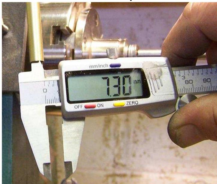
**Now the fun part!!! Hold a good clean file in the LEFT HANDED method and with the lathe on quite slow, go for it. Stroke the file left to right in smooth circles. It goes pretty quick so keep checking with the calliper. Use a sharpie to mark any high areas. As the file does not leave the surface, you don't have to worry at all about the washers. Use chalk on the file to prevent clogging and rip out. ( I can't touch chalk, so I just use a wire brush to keep the file clean)**
