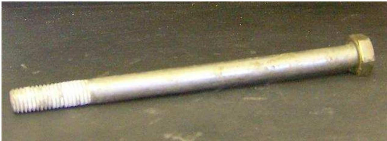
**Now cut the hex head off with a hacksaw in a vice and square up the end with a file on the lathe.**
