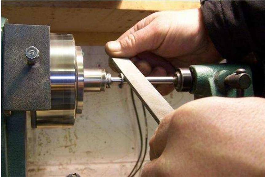
**Once the caliper goes over the bolt throughout its length, you can remove the tailstock. Now change to about 240 grit wet'n'dry and use it to get the brass tube to fit as snug as you can. Use the sharpie and start from the end. It should look like this.**
