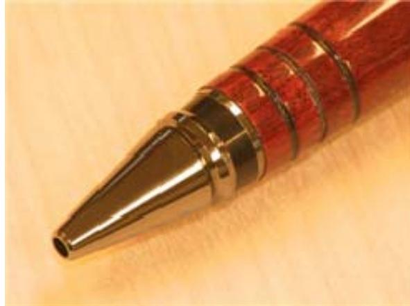
When you press in the tip, use epoxy to fill the gap to give the tip mechanical strength. The end result does not look too shabby (picture 31), even though I was not careful enough with the diameter, and this pen, because of the epoxy to wood joint, is not a good candidate for disassembly.
