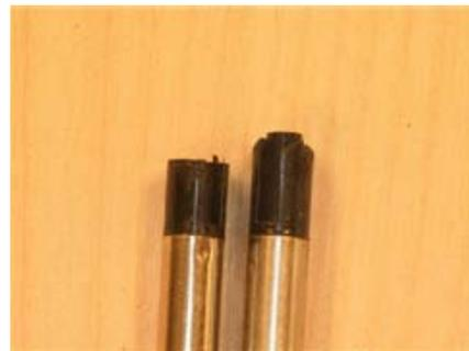
should be the first line of defense because it's the simplest. Similarly, on a Cross-type refill, you can pull off the black cap and shorten the metal tube, if for some reason you can't or don't want to adjust the mechanism.
