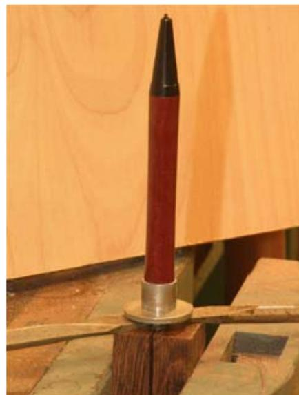
To protect the pen barrel from the prying screwdriver a bushing and a washer are used (see picture 1). The refill
