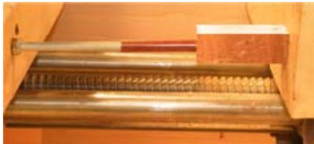
variation of that is a size D (0.246") or even 1/4" hole dilled in a piece of hardwood. The hole just fits the transmission, but catches the barrel. A 1/4" bolt can serve as push rod. Picture 2 shows the home-made 'kit', and picture 3 shows it being used in a bench vise.
