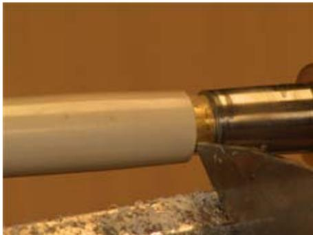
I start by parting off enough of the damaged area to have a clean face (picture 16). The shoulder of the face should be square or have a small undercut so a piece can be added without gap. I have a box of cut-offs from pen blanks and can usually find something suitable. Here I use the same material as the original.
