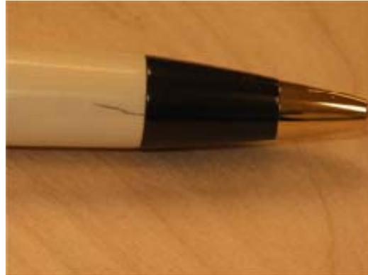
Picture 15 shows a crack that developed after assembly in a piece of mammoth ivory, because I was careless and did not file out the brass tube sufficiently to let the fitting slip in. In this case I added a piece of ivory, and hid the joint under a ring of crushed stone.
