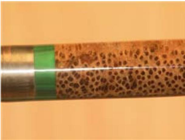
blended it in with the wood, another chunk of wood came out, right next to the previous repair! See picture 22. Again I simply filled with sawdust and CA (picture 23). The final repair is nearly invisible (picture 24). Often you can also orient the clip to hide a repair that does not blend in quite as well.
