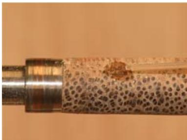
CA, because it wicks in best. I immediately follow it with a drop of medium CA to fill some of the gaps better. It's best to allow this to air dry and not hit it with accelerator to avoid frothing. The accelerator starts a reaction that heats up the CA, and because of the large local concentration it generates enough
