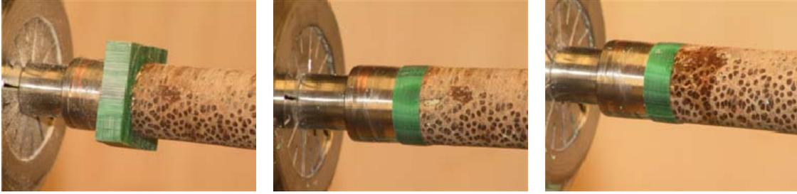
Some wood had broken out at the end. Again I cut a tenon and add a piece of contrasting material, trustone in this case (picture 21) After turned it to size and
