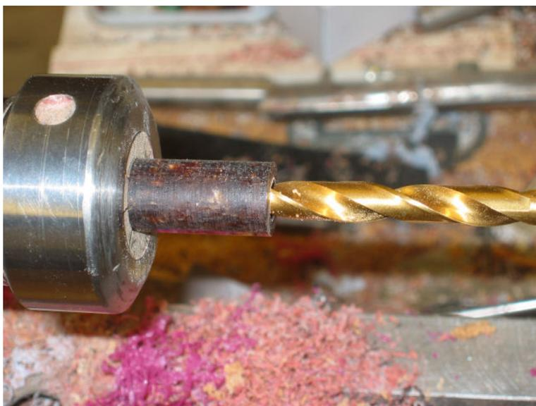
After drilling, support the end with a center and turn to size for a slip or press fit in the cap tube. I prefer a slip fit and a little epoxy, then I don't have to work quite as precisely ☺
