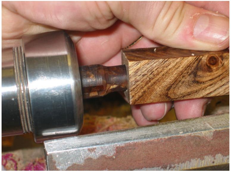
Here is the spacer ring on the loose center coupling. There is very little space where the section protrudes from the cap fitting – excellent. The second picture shows another ring, this time with the coupling in the closed position. So now a little epoxy is applied inside the cap tube where the spacer will sit. The spacer is inserted first, then the center coupling pushes it up into its final position
