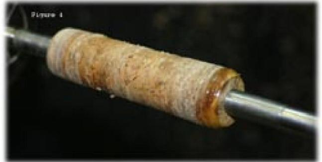
**Figure 5:** Removal of the excess slurry with round nose scraper or the tool of your choice.
