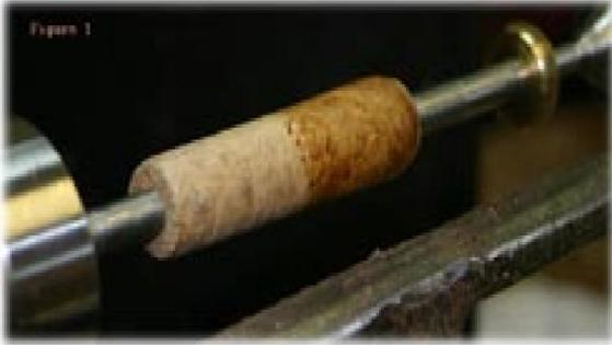
**Figure 2:** Collecting sanding dust with 180 grit to use for the CA slurry as a sealer. This step could be omitted and a sanding sealer used. The slurry works exceptionally well for open grain woods.
