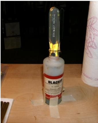
Now take your cleaned tube and dunk it into the bottle of oxidizer. The reason I use an awl is that it rests nicely on the bottle neck; however, using a piece of dowel rod works just as well - just let it rest on the bottom of the container (make it long enough to act as a retrieval "handle" sticking out of the bottle).
